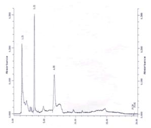
Figure 6 b - DCM HPLC spectrum
